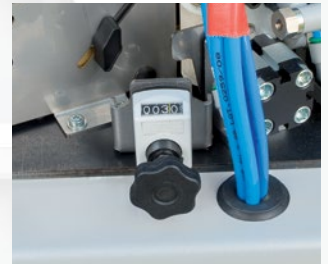
Simultaneous adjustment for the tape thickness, intake guide and gluing roller by a single digital meter.
