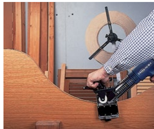
Enables banding of circular or shaped pieces.
