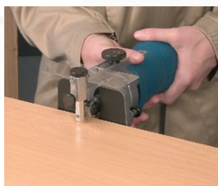
Excellent finishing when trimming laminates.
