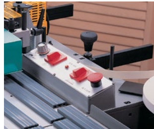
Safety control (STOP). Electronic temperature control.
