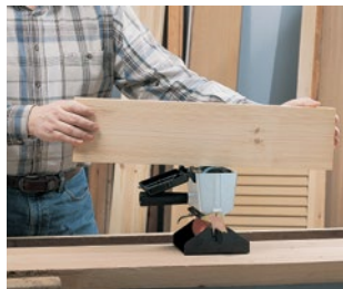
Gluing with the upper roller.
