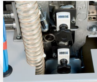
Direct adjustment of the trimming bits and copiers by digital meters.
