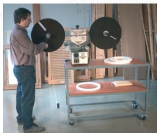
Easy to handle and start, allows rolls to be preglued without complications.
