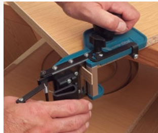
Cutting on both sides on straight panels.
