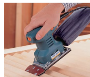
Sanding difficult to reach areas such as blinds, etc...
