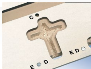
Cross form trimming for jointing both sides of work top.
