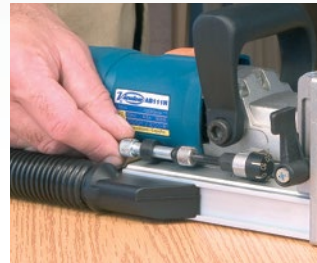
Quick adjustment of different slotting depths.
