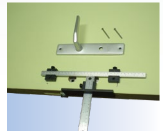
Drilling for door accessories.
