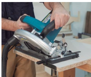
Performs cuts of up to 75 mm.
