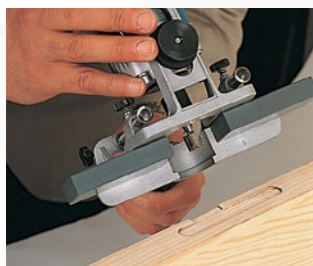
Placing hinges with the ZB93 head.
