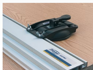
The guide can be fixed by means of the two suction pads included (on smooth and non-porous surfaces).
