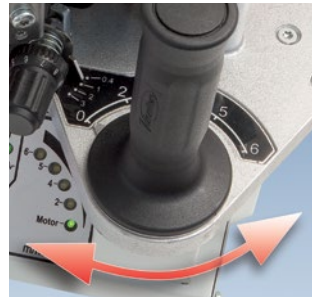
Speed adjustment controlled by microprocessor.
