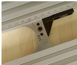
Equipped with a special stopper for a 90° trimming.
