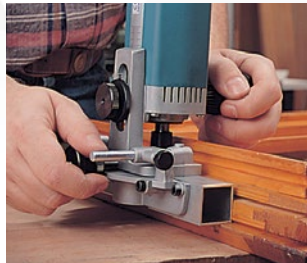
Slotting a window, flashing side.
