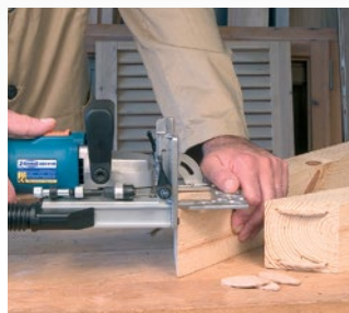
Stronger joints with No. 6 splines.
