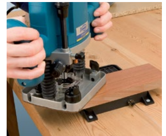
Securing small pieces on a divided portion of the suction plate.
