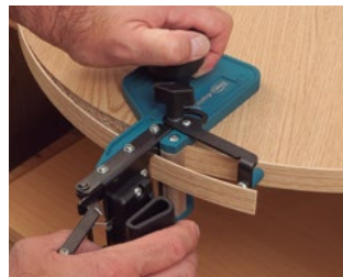
Cutting on circular panels.
