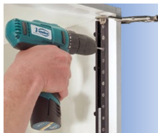
Drilling for placing shelves.
