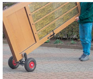
Allows just only one person to hold and carry all kind of panels, heavy doors.
