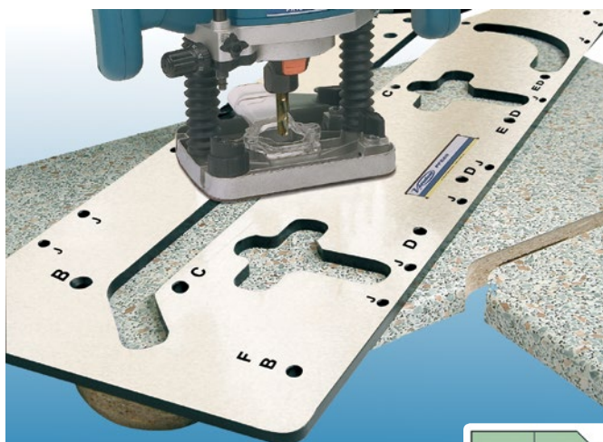
Cross form trimming for jointing both sides of work top.
