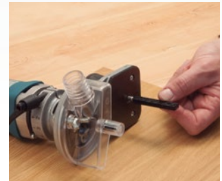
Precise guiding for corner trimming.
