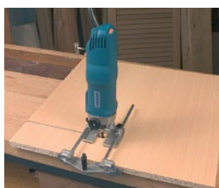
Trimming parallel slots.
