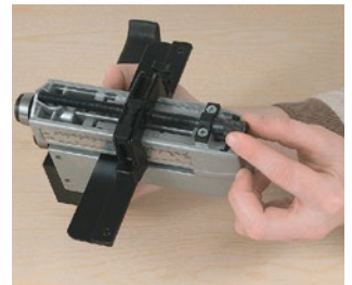
Micrometric regulation of the cutting width.
