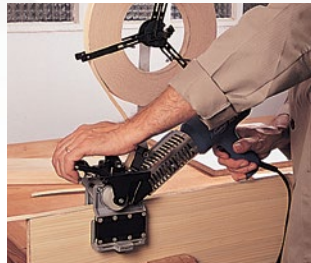
High precision and stability during edgebanding.
